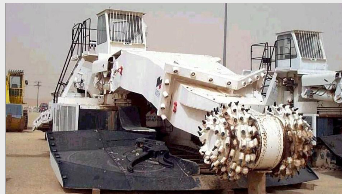
Figure 4-24 Roadheader Excavation Machine
