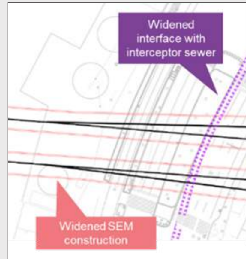
Figure 5-5 Interface with Twelfth Avenue Interceptor Sewer
