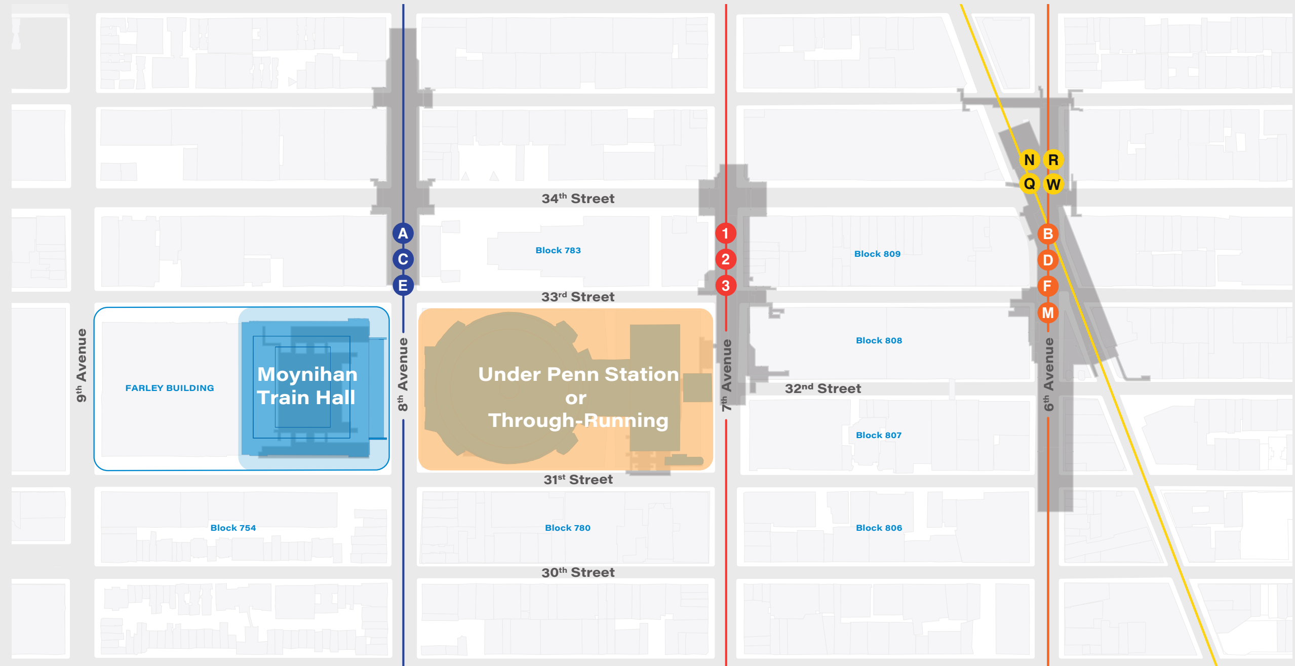
Figure 1-3 Two alternatives for maximizing rail capacity at Penn Station within the existing station footprint
